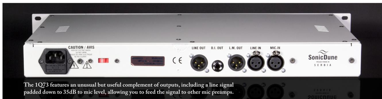
The 1Q73 features an unusual but useful complement of outputs, including a line signal padded down to 35dB to mic level, allowing you to feed the signal to other mic preamps.
